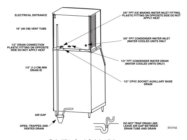
**Typical Water Supply Drain Installation**
